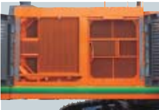
Radiator and Oil Cooler Designed for easy cleaning.
