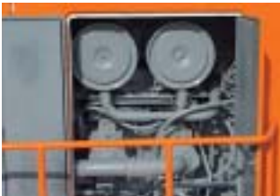
Dust Ejector Automatically Airborne dust and particles are separated/ejected automatically, extending element cleaning and replacing interval.
